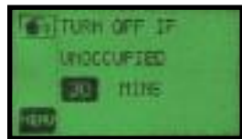
Occupancy Sensor automatically turns off the air conditioner when the room is unoccupied
