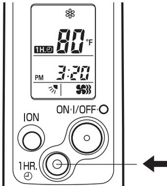
This function causes the unit to operate for one hour and then stop, regardless of whether the unit is on or off when this button is pressed. The **1HR.Ⓢ** indicator in the display indicates that this function is operating.
