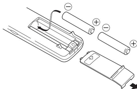
1. Slide the cover in the direction indicated by the arrow and remove it.
