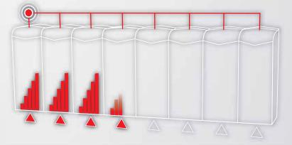
Cascading continues as additional boilers fire in sequence, until all units are in operation or demand is satisfied. When demand drops, the cascading process reverses, with the precision, control and performance you expect from Lochinvar.
