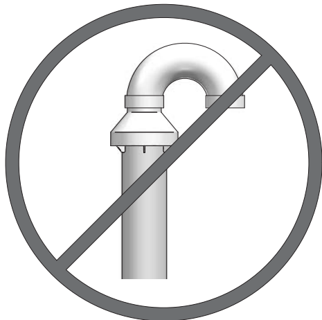
Figure 5-6 Do Not Install U-Bent to Rain Cap
