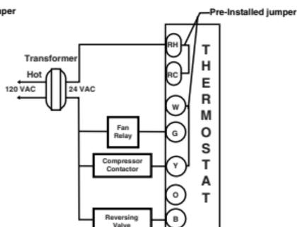
NOTE: Installer must place jumper between W and Y terminals.
