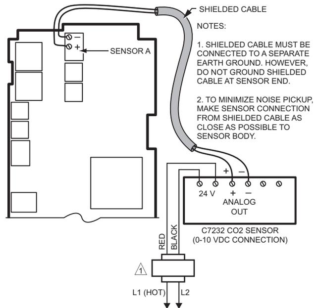
⚠ USE SEPARATE 24 V TRANSFORMER TO POWER THE C7232 CO<sub>2</sub> SENSOR. PROVIDE DISCONNECT MEANS AND OVERLOAD PROTECTION AS REQUIRED.
