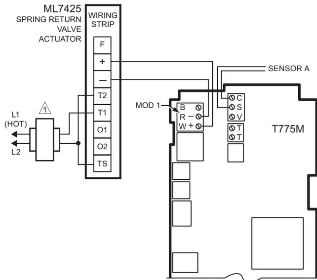
⚠ POWER SUPPLY. PROVIDE DISCONNECT MEANS AND OVERLOAD PROTECTION AS REQUIRED.
