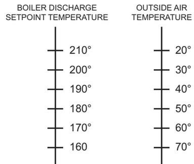
Fig. 28. Boiler Discharge Temperature vs. Outside Temperature.
