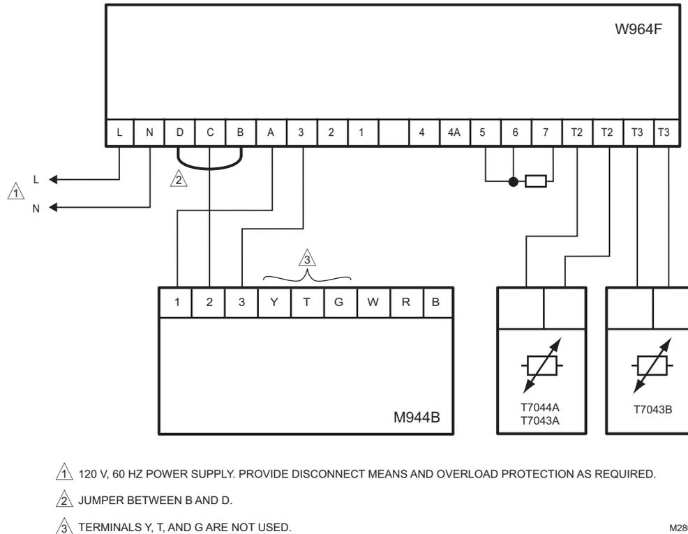
**Fig. 36. W964F Wiring Connections (Pre-existing Control).**
