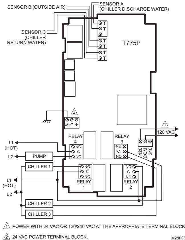
**Fig. 24. T775P Wiring - Multi-Stage Chiller Control (No Reset).**
