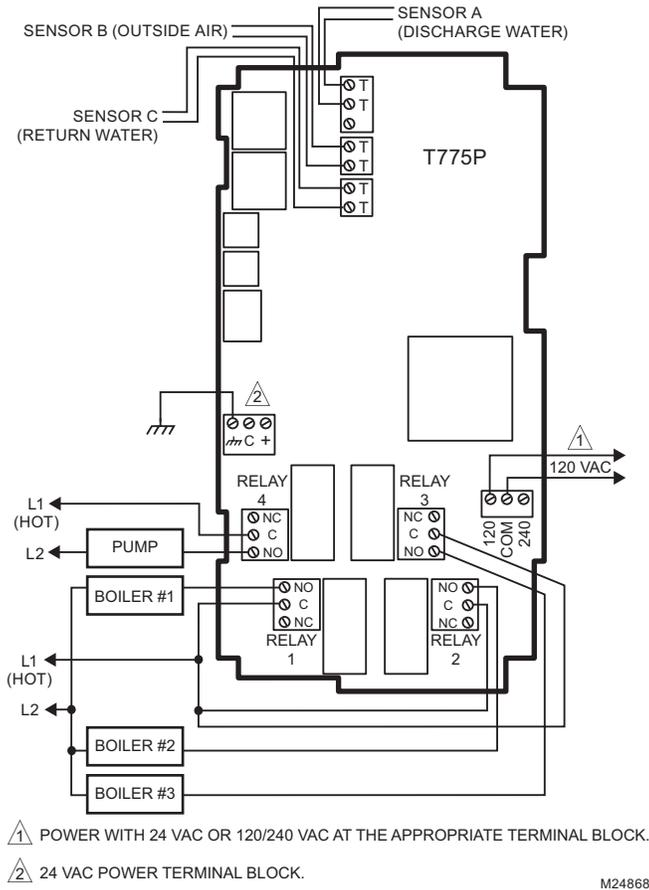
Fig. 22. T775P Wiring - Multi-Stage Boiler Control with Reset.
