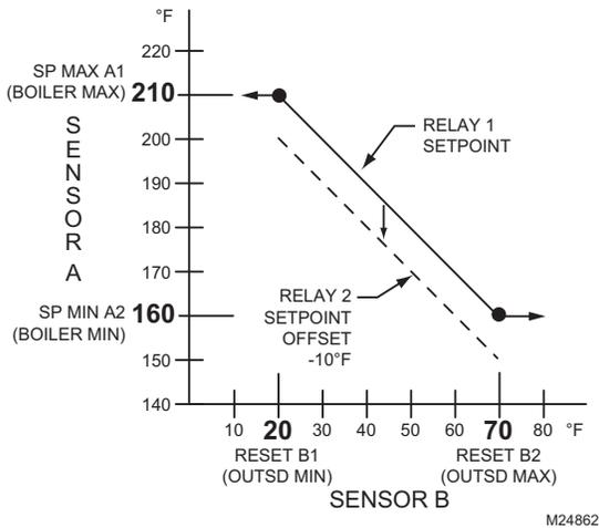
Fig. 1. Reset Curve with Offset for Subsequent Outputs.
