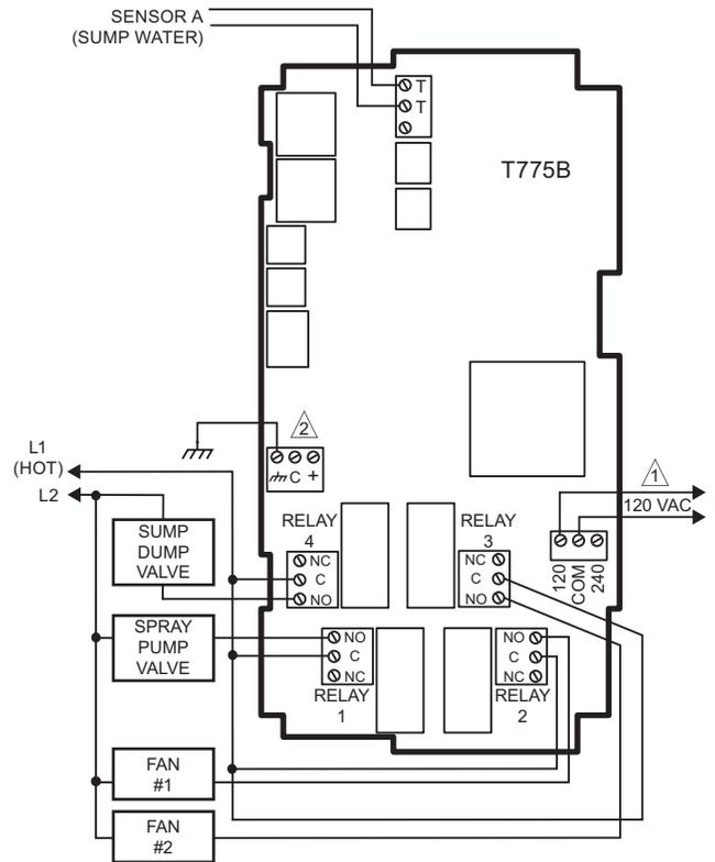
⚠ POWER WITH 24 VAC OR 120/240 VAC AT THE APPROPRIATE TERMINAL BLOCK.
