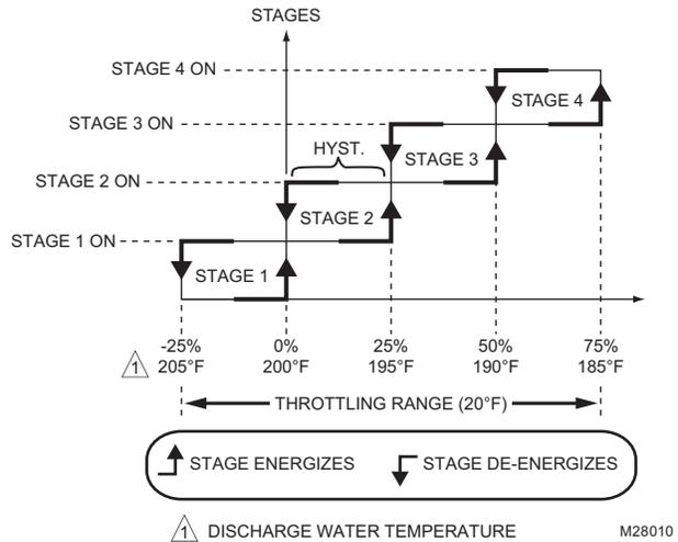
**Fig. 25. Staging Behavior (when the effective setpoint = 200° F (93° C))**
