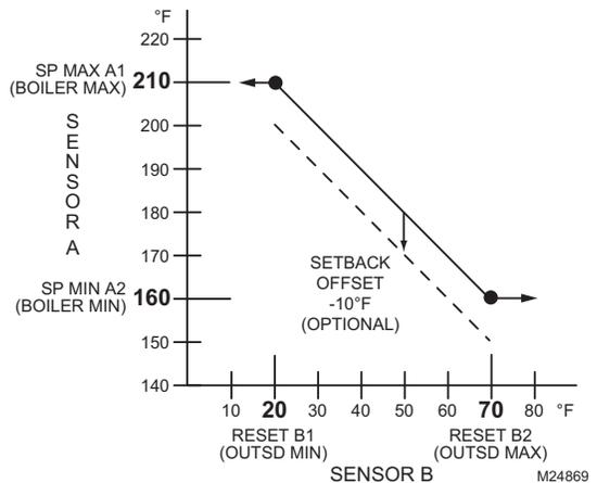
Fig. 21. Reset Curve with Optional Setback Offset.
