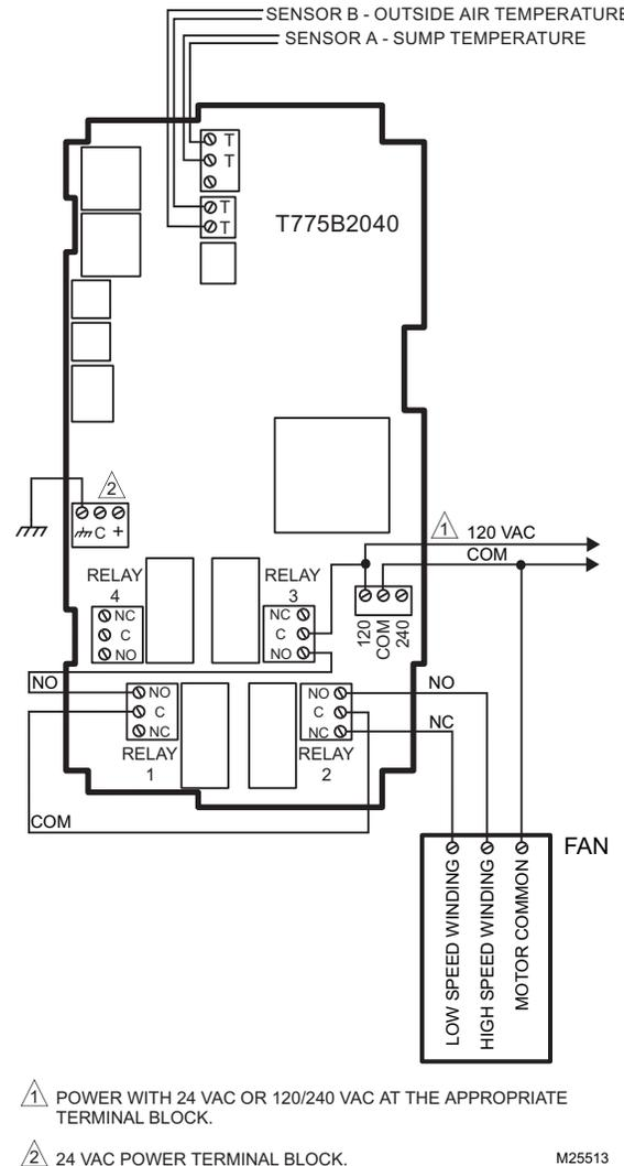
Fig. 6. T775B2040 Wiring for Cooling Tower Control.
