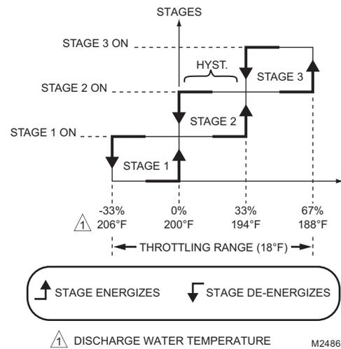
Fig. 18. Boiler Control Staging Behavior (when the effective setpoint = 200° F).
