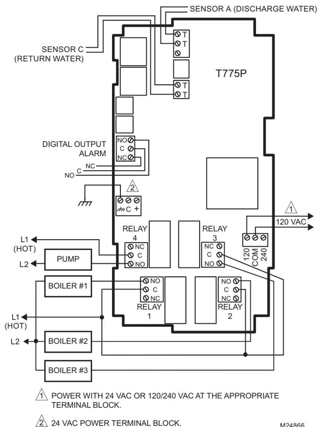
1 POWER WITH 24 VAC OR 120/240 VAC AT THE APPROPRIATE TERMINAL BLOCK.
