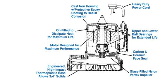
The Model 10E Series De-watering and Effluent pumps are for commercial and light industrial applications. Pumps feature a 1-1/2" discharge, with a lift of 26', ABS base, vortex nylon impeller and glass-filled electrical case.
