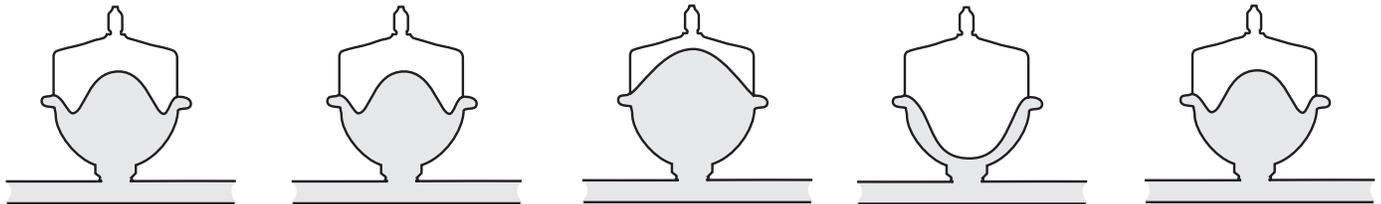
1. When water in the house is not being used, the 150A is in its normal state, where the air charge and water pressure do not flex the diaphragm.
