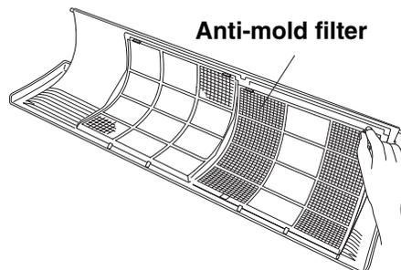
**Cleaning** Use a vacuum cleaner to remove light dust. If there is sticky dust on the filter, wash the filter in lukewarm, soapy water, rinse it in clean water, and dry it.
