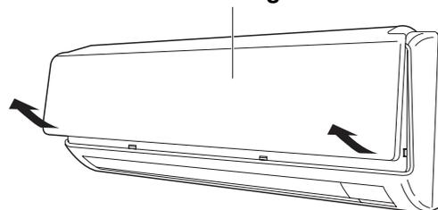
2. Remove the anti-mold filter attached to the rear of the air intake grille.
