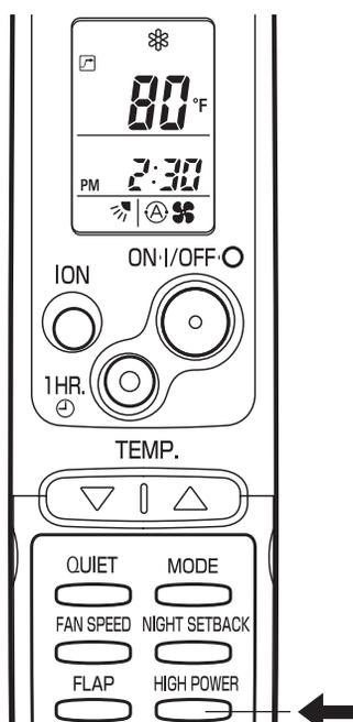
HIGH POWER mode can be used to increase the output of the indoor unit for all operation modes.
