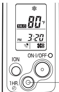
This function causes the unit to operate for one hour and then stop, regardless of whether the unit is on or off when this button is pressed. The **1H.** indicator in the display indicates that this function is operating.
